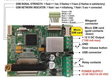
\*<u>Do not use the 12V AUX power output for electric lock driving!</u>
